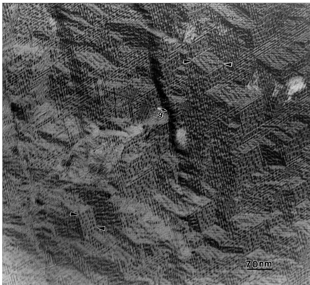
Fig. 2. Bright field image taken in nearly two beam condition showing the linear fringe type contrast perpendicular to g_p vector. Rhombic domain has been indicated (arrowheads).
